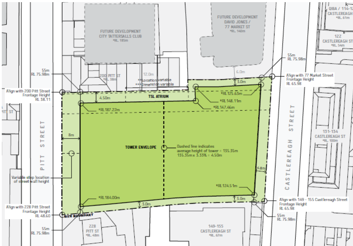
Figure 17. Setbacks of the indicative building envelope
